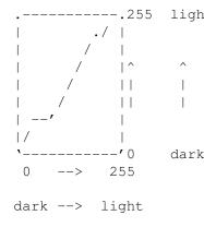
> This deviation depends on the electronical and dark optical calibration of the scanner hardware. With a color look-up table is is possible to compensate this deviation. The Look-Up Type "Gamma" leads normally to the best results. You should test various gamma values to get the best curve for your scanner.
